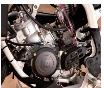
TWO STROKE. Small cylinder unit, ultraslim cylinder head, carburettor with base gasket on the casing: unequivocally 2stroke.... with HTS dual shutter valve on the exhaust and V Force 3 valve group with double reed petals.
